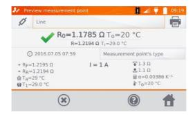
The printout includes all the results and parameters of the measurement, assessment (positive/negative), the date and time of measurement and data of person performing it, entered in the printer settings.
