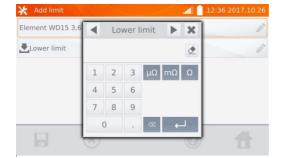
Enter the lower limit. Use button to go to the upper limit setting. You can also set only one of the limits.
