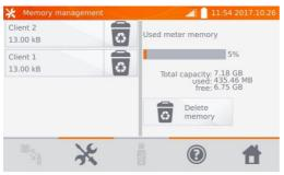
This option allows you to read the % of the used memory and to clear it: after clicking **Delete memory** all clients are deleted with their objects and measurement results. By pressing button customer, you can also delete individual customers.
