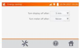
Set the inactivity time for blanking the screen and turning off the meter.
