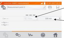
When measuring inductive objects, only Auto mode is available - the measuring current is limited to a value not exceeding the set value,
