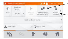
Switching Unidirectional/Bidirectional measurement.
