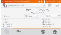
8 Connect the meter to the tested object. Press START/STOP.
