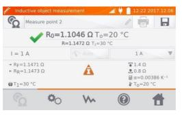
After the measurement or before ir, click **Measurement point name** and enter the name.
