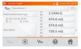
When using the logger, clicking the field with results will cause the meter to display the individual samples. You may scroll them using , buttons. Use button to display the graph.
