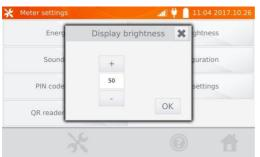
Use "+" and "-" buttons to set the desired brightness and confirm it by pressing **OK**.
