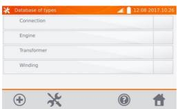
The meter has 4 default types saved in its memory. Use to button to add a new type of the tested object.
