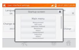
Click the selected startup screen (the screen will be automatically shown after turning on the meter). This feature is useful for making measurements of a given type for a longer period.
