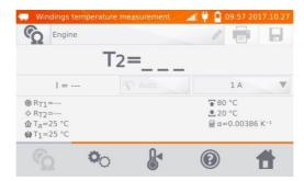
(8) Connect the meter to the motor windings. Press START/STOP.
