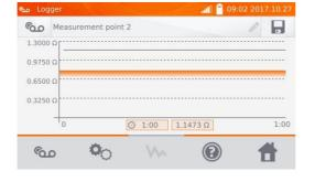
Use who button to display the graph of resistance over time - both during the logging process and after its completion.
