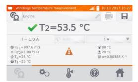
R<sub>T1</sub> – resistance of the cold winding
