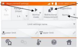
Switching Unidirectional/Bidirectional measurement.
